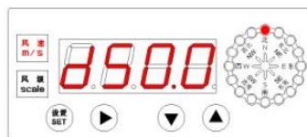
Fig. 5: wind speed range setting
