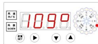
Fig. 6: Wind direction setting
